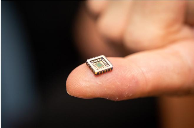
One of the artificial neurons in its protective casing on a fingertip. Credit: University of Bath
