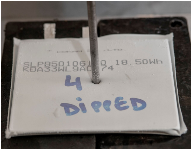
A frozen battery cell with a nail through it. Credit: University of Warwick
