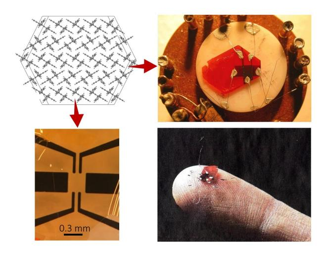
Organic transistors based on single crystals of rubrene, a hydrocarbon, can roughly double the speed of electricity flowing through them when a crystal is slightly bent (strained). This useful behavior cannot be easily achieved with traditional semiconductors made, for example, of silicon. Molecules of rubrene are arranged in a herringbone pattern (upper left), forming highly ordered semiconducting molecular crystals that can be used to create rigid (upper right)
