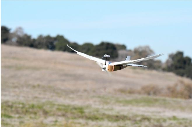
Researchers at Stanford University said they had studied the wings of common pigeon cadavers, then used their findings to build a radio-controlled robot with wings made with 40 real feathers
