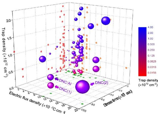
3D scatter plot of transistor bias-stress data taken from previous literature. Credit: Lin et al.
