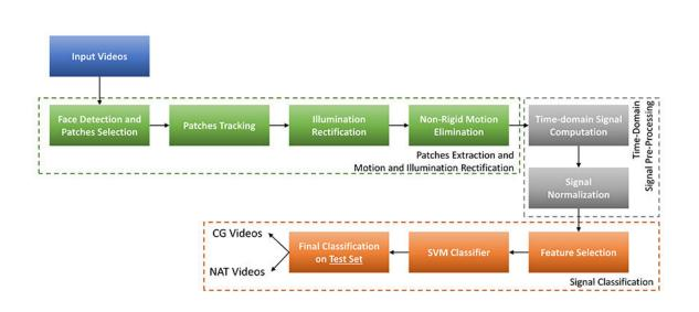
Algorithm process flow. Three main phases characterize the workflow: (a) temporal signal computation from face patches and denoising; (b) signal normalization; and (c) feature extraction and SVM classification. Credit: Bonomi and Boato
