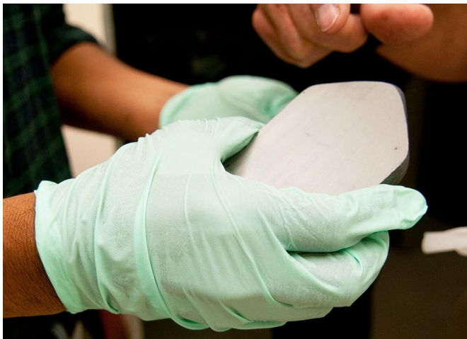
A sample crystal of cadmium telluride material that can be used to make solar cells. Credit: WSU
