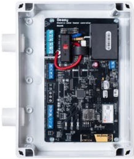
An electric water heater controller. Provided by author.
