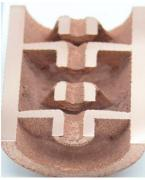
Examples of 3D-printed copper components that could be used in a particle accelerator: X-band klystron output cavity with micro-cooling channels (at left) and a set of coupled accelerator cavities. Credit: Christopher Ledford/North Carolina State University
