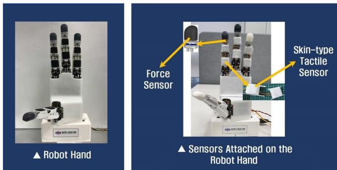
Tactile Sensor-integrated Robot Hand. Credit: Korea Institute of Machinery and Materials (KIMM)
