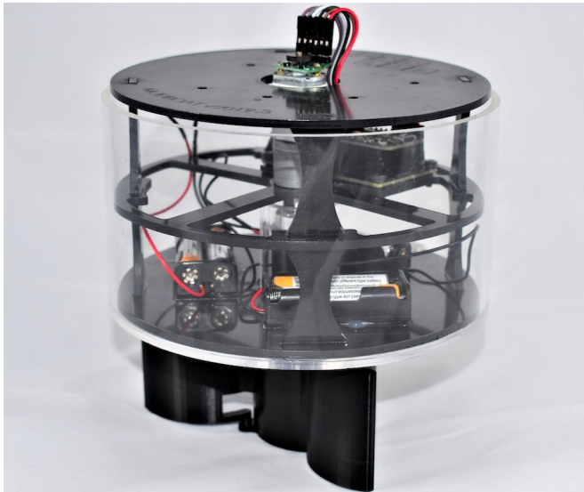
Modboat: The low-cost robotic boat created by the researchers. Credit: Knizhnik & Yim.
