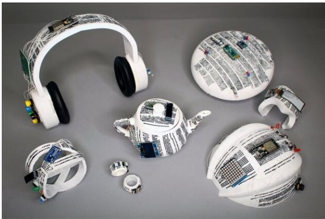
CurveBoards are 3D breadboards — commonly used to prototype circuits — that can be designed by custom software, 3D printed, and directly integrated into the surface of physical objects, such as smart watches, bracelets, helmets, headphones, and even flexible electronics. CurveBoards can give designers an additional prototyping technique to better evaluate how circuits will look and feel on physical products that users interact with. Credit: Dishita Turakhia and Junyi Zhy
