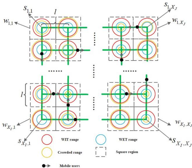
Figure illustrating the smart city environment considered by the researchers' H-AP deployment scheme. Credit: Zhao et al.
