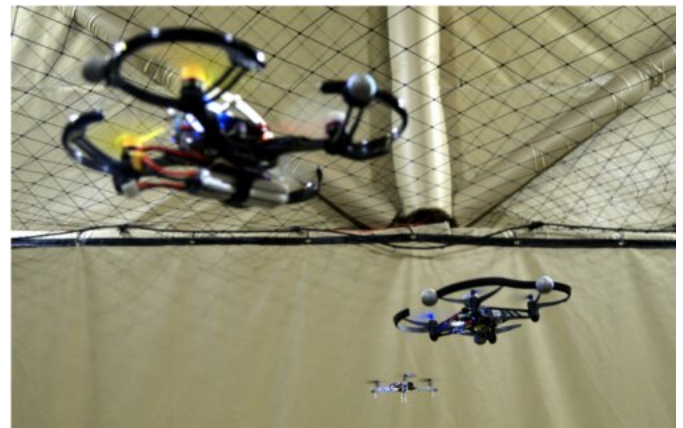
Three quadcopters of different sizes controlled by the same policy trained entirely in simulation. Credit: Molchanov et al.
