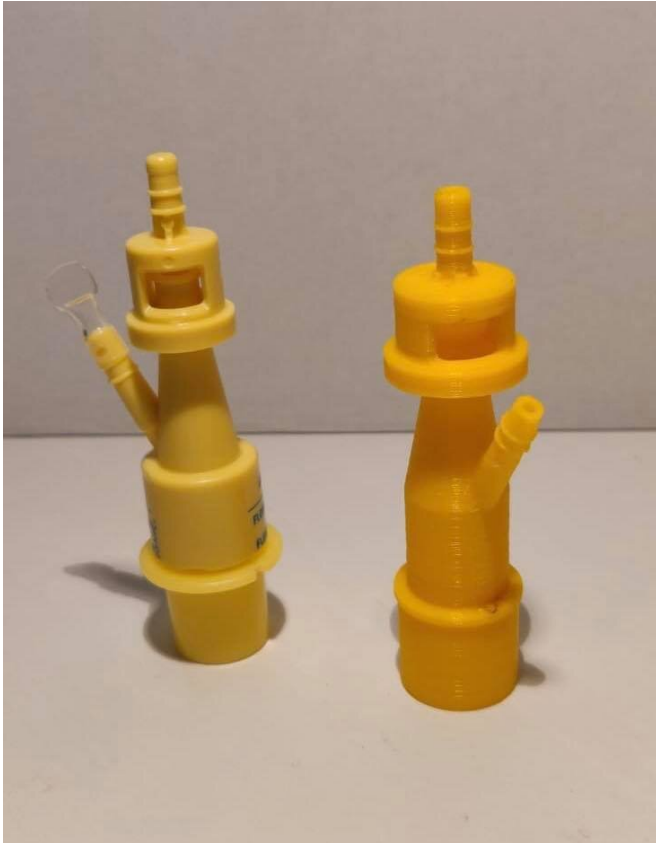
The original valve (left) and its 3-D printed twin. Credit: Cristian Fracassi
