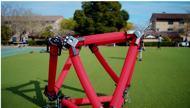
After inflation, the isoperimetric robot can move and transform untethered to a power or air source. Credit: Farrin Abbott
