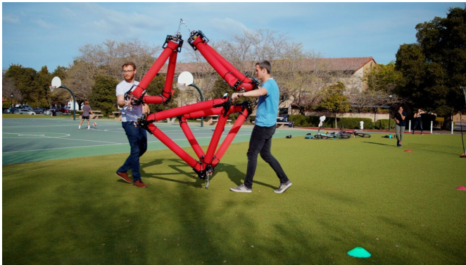
Graduate students Zachary Hammond (on left) and Nathan Usevitch pick up and move the isoperimetric robot, demonstrating that it is lightweight, resistant to damage and safe around humans. Credit: Farrin Abbott
