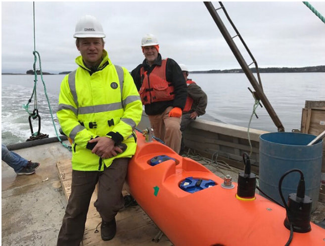
Levi Kilcher and Bob Lewis prepare to launch the StableWing ocean-turbulence measurement platform in the Western Passage of Maine. Credit: Levi Kilcher, NREL
