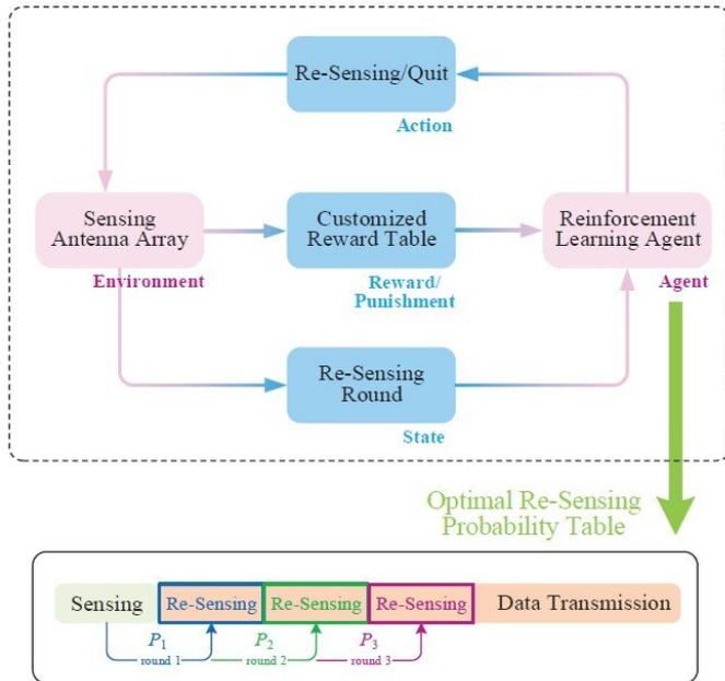
Reinforcement-learning-driven automatic repeat sensing mechanism. Credit: SARI
