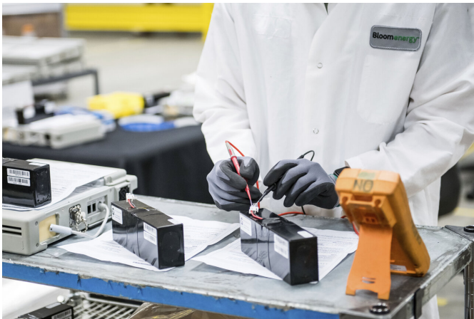
In this March 28, 2020, file photo, David Yee, an NPI mechanical engineer, tests voltage of new batteries at Bloom Energy in Sunnyvale, Calif. The COVID-19 outbreak has prompted companies large and small to rethink how they do business. Bloom Energy makes hydrogen fuel cells. But recently, they have been refurbishing old ventilators so hospitals can use them to keep coronavirus patients alive. (Beth LaBerge/KQED via
