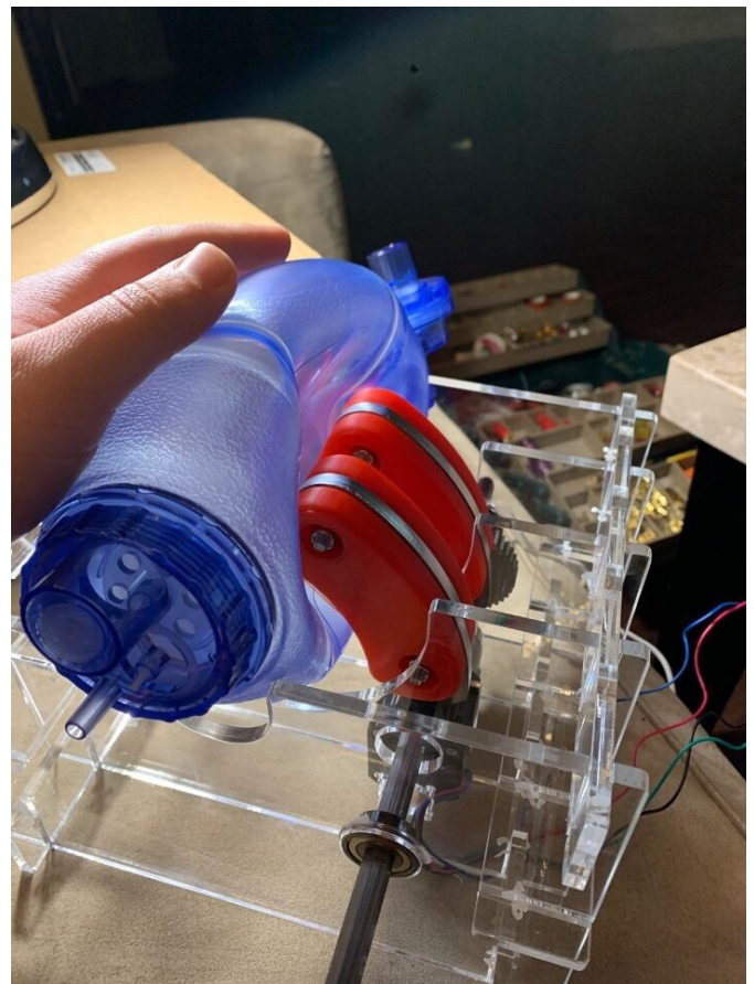
Single arm AMBU-bag compression design build. Credit:
