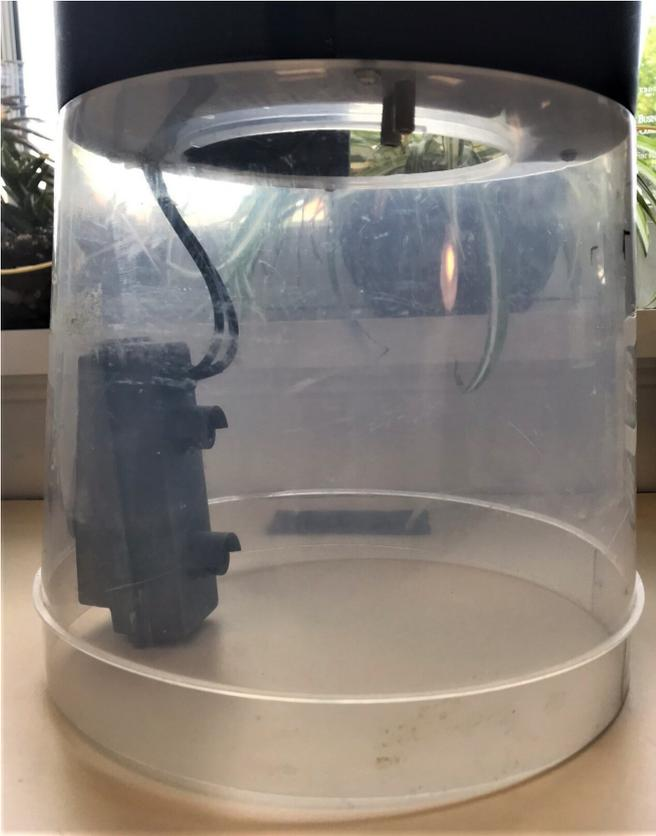
A new low-cost imaging system for monitoring mosquitoes could be used to transmit images of mosquitoes inside traps like the one seen here. This could make it easier to track mosquito species that carry disease. Credit: Adam Goodwin, Johns Hopkins University
