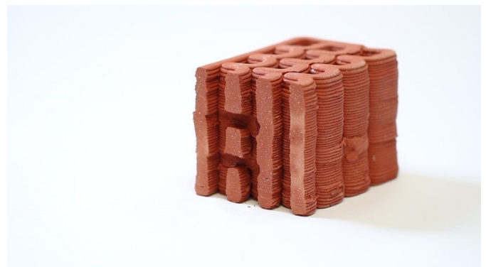
cold-SNAP creates a ceramic-based heat exchange unit
