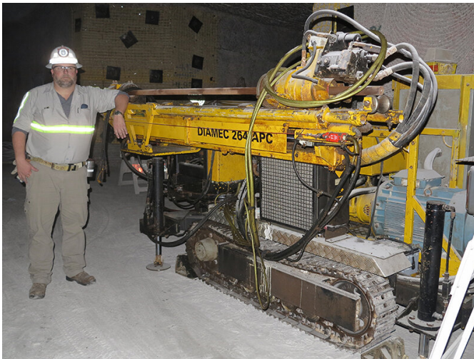
Doug Weaver, also on the BATS research project, stands by one of the large drills used to create the boreholes for experimentation. Credit: Brian Dozier
