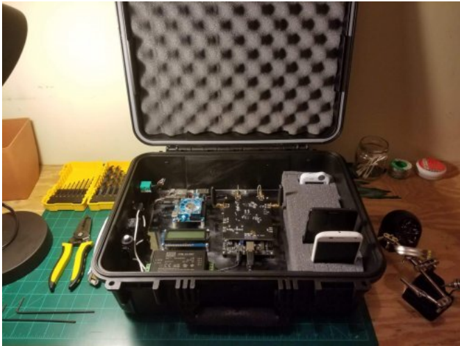
Inside the Beamlink case: a cellular base station, test mobile phones and a portable EKG device. Credit: Arpad Kovesdy
