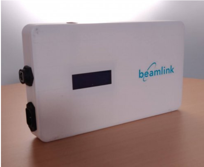
The newest 3d-printed prototype of Beamlink's portable cell tower. Credit: Mateo Abascal
