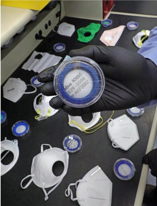
The SwRI Particle Science and Technology Laboratory team is testing N95 and KN95 respirators and surgical masks for quality assurance. Engineers cut out a sample of mask material to evaluate particle filtration and flow resistance. The team previously focused solely on engine emission particle testing. They began testing mask materials for health care, government and industry clients in response to the COVID-19 pandemic. Credit: Larry Walther, SwRI
