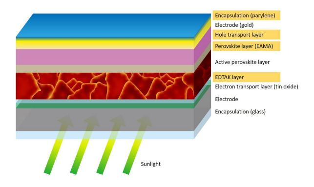
Perovskite solar cells and modules consist of many layers, each of which has a specific function. The scientists added or modified the layers highlighted in orange. Credit: OIST
