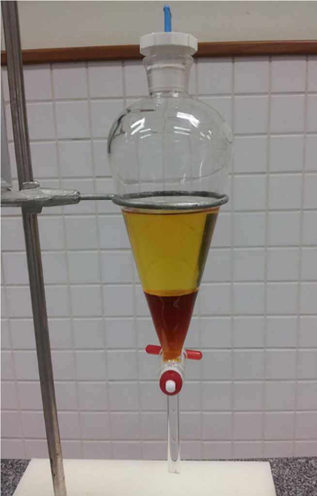
The two-phase system containing biodiesel (upper phase) and glycerol (lower phase) Credit: Gilberto Maia de Brito
