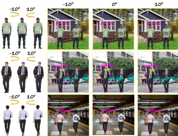
Examples of the researchers' 3D adversarial logo attack using different 3D object meshes, with the aim of fooling a YOLOV2 detector. Credit: Chen et al.
