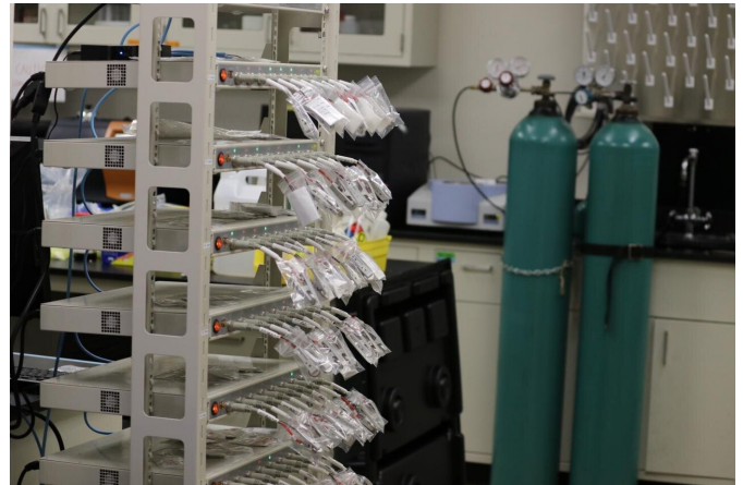
Battery testing system in Dr. Yu's Lab for developing advanced electrode materials. Credit: The University of Texas at Austin
