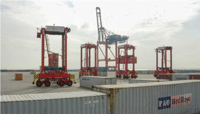
Automated straddle carriers at the container terminal in Wilhelmshaven – efficient and secure. Credit: EUROGATE
