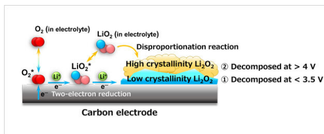
Figure. Schematic diagram illustrating the two Li 2 O 2 formation pathways during a discharge cycle in a lithium-air battery. Credit: National Institute for Materials Science
