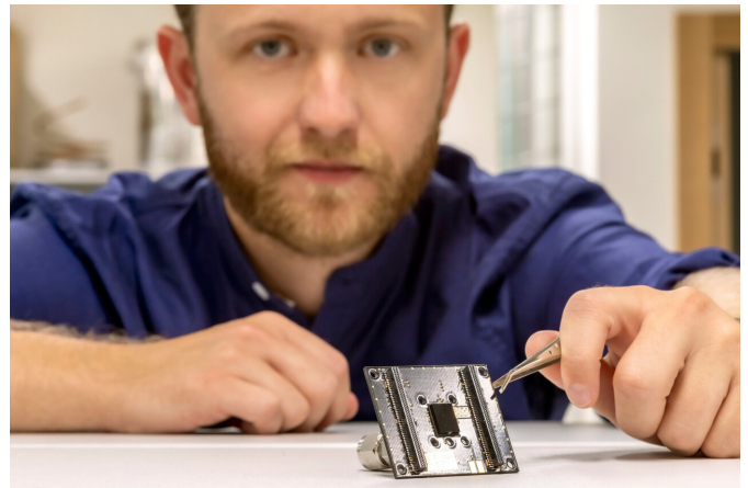
Paul Maierhofer with the result of his dissertation at the Institute for Electrical Measurement and Sensor Technology at Graz University of Technology: the 12 x 9 x 3 millimetre small particle sensor. Credit: Lunghammer - TU Graz
