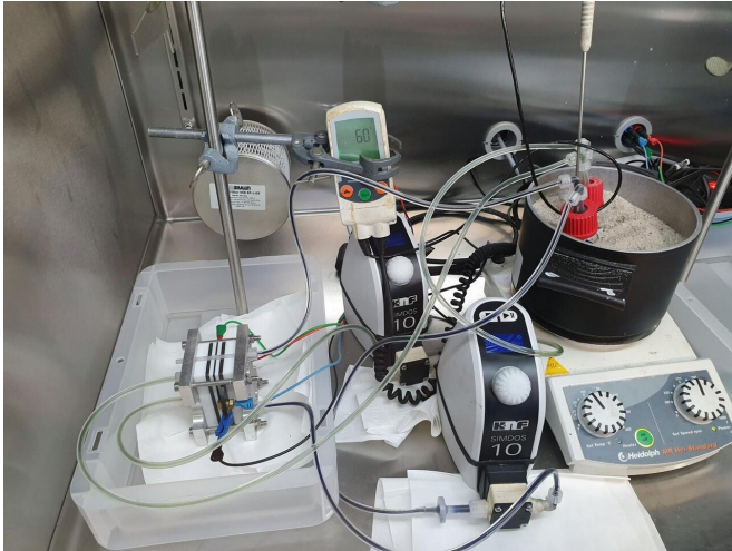
Test setup at CEEC Jena to develop novel active materials for redox flow batteries. Credit: Philipp Borchers/University of Jena
