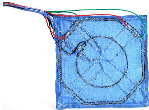
Top-down image of a robotic fabric with integrated actuation, variable stiffness, and sensing fibers. Credit: Rebecca Kramer-Bottiglio
