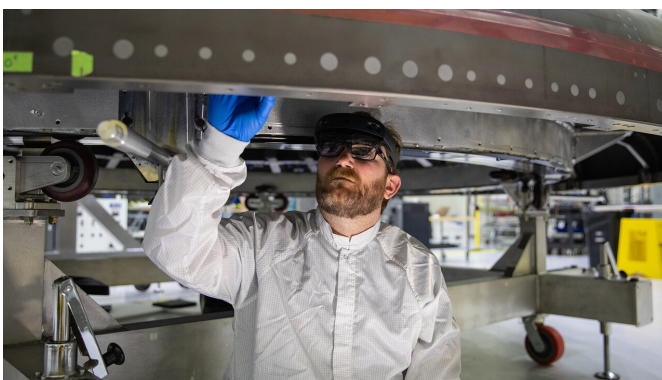
Eric Nolan, a technician working at the Kennedy Space Center, wears a HoloLens2 as he works on the heat shield for the crew module for NASA's Artemis II
