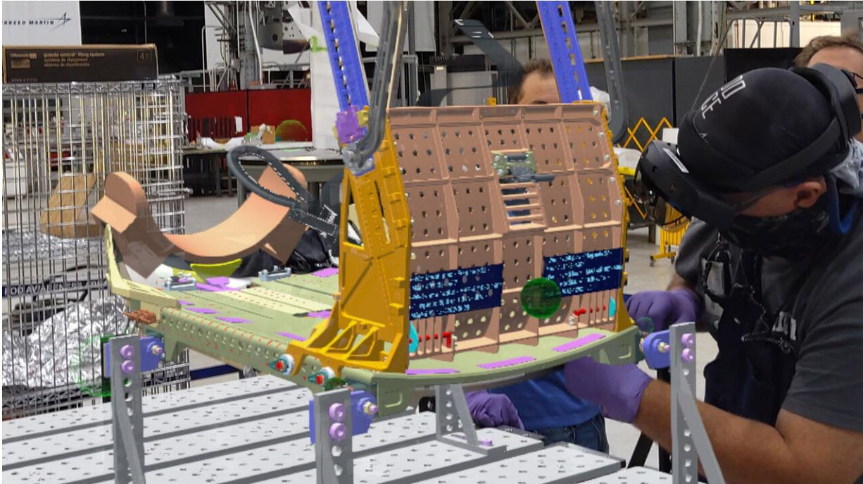
Lockheed Martin technicians at the NASA Michoud Assembly Facility use HoloLens 2 to assemble Orion's crew seats for the Artemis II mission. This image, captured with a HoloLens 2 headset, shows the holographic instructions overlaid on the crew seats. Credit: Lockheed Martin
