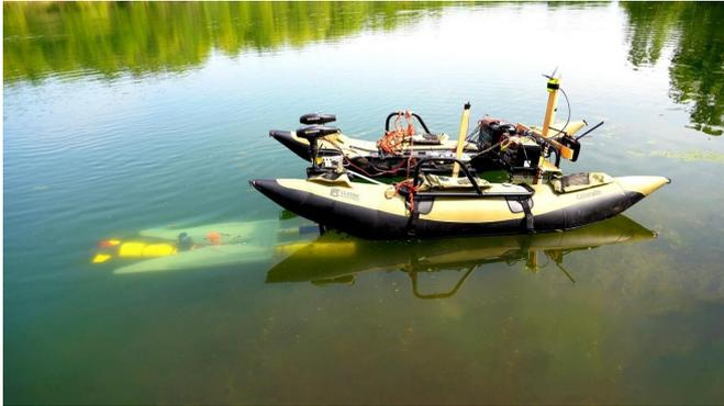
A yellow underwater robot (left) finds its way to a mobile docking station to recharge and upload data before continuing a task. Credit: Purdue University photo/Jared Pike
