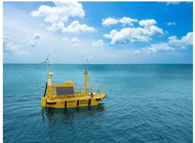
U.S. Department of Energy lidar buoy deployed off Morro Bay, California. Credit: AXYS Technologies and PNNL
