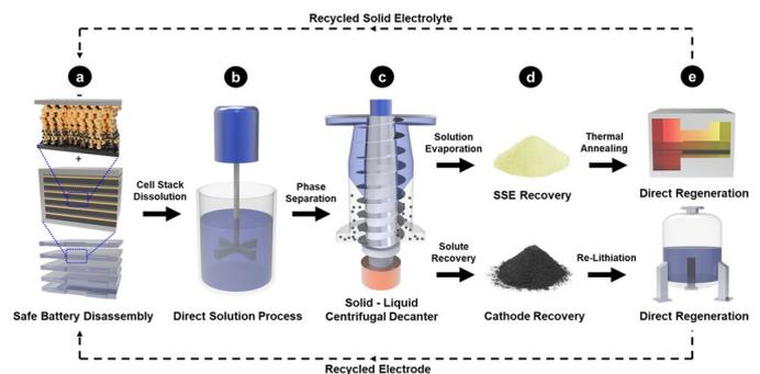
A proposed procedure for recycling solid-state battery packs directly and harvesting their materials for reuse. Credit: [Tan et al., 2020, CC BY](#)
