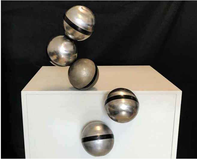
A freeform MSRR system - FreeBOT. Credit: Guanqi Liang et al.
