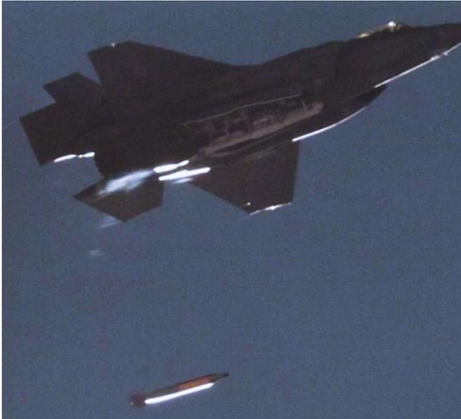
An F-35A Lightning II opens its bomb bay doors and drops a mock B61-12 at Sandia National Laboratories' Tonopah Test Range. Credit: Sandia National Laboratories
