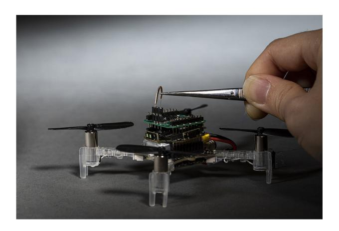
By adding tiny wires into either end of the antenna (the arc being attached here), the researchers were able to connect it to a circuit and record its responses. Credit: Mark Stone/University of Washington
