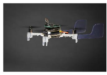
Smellicopter has two plastic fins (shown here in blue) on the back to create drag to help it be oriented so that it is constantly facing upwind. Credit: Mark Stone/University of Washington
