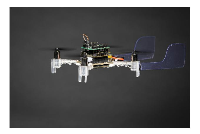
Smellicopter has two plastic fins (shown here in blue) on the back to create drag to help it be oriented so that it is constantly facing upwind. Credit: Mark Stone/University of Washington
