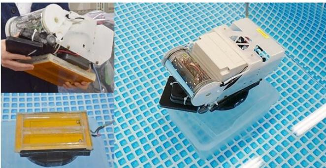
Underwater drone (top left), power supply station (bottom left), drone parked on the power supply station installed on the ocean floor for battery charging (right) Credit: Toyohashi University of Technology.
