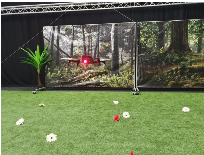
Drones can use oscillations to perceive their distance to objects. Here the drone is learning to detect and avoid obstacles in our experimental flight arena. Credit: MAVLab/ TU Delft
