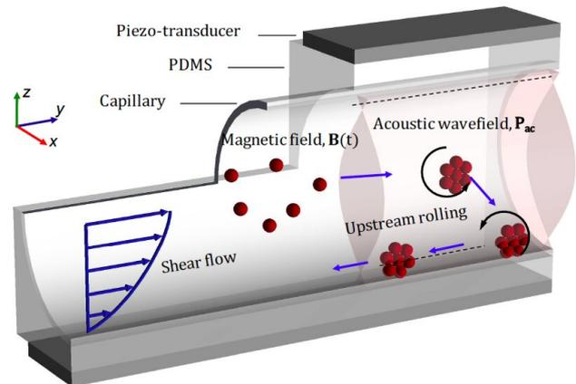
In a bioinspired system, superparamagnetic particles injected into the capillary self-assemble into a spinning microswarm due to the dipole–dipole interaction of a rotating magnetic field. The microswarm was shown to be marginalized towards the wall due to the presence of acoustic pressure nodes (marked as dashed black lines). Image 1: Credit: Ahmed et al.
