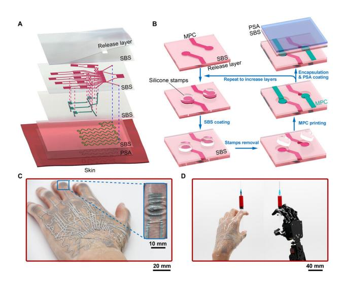
Schematic illustrations and optical images of the three-layered METT. (A) Exploded schematics of the METT containing three circuit layers. (B) Schematic illustrations of the layer-by-layer fabrication of the METT. (C) Optical image of the METT after transferring onto the skin; inset, the METT can be embedded
