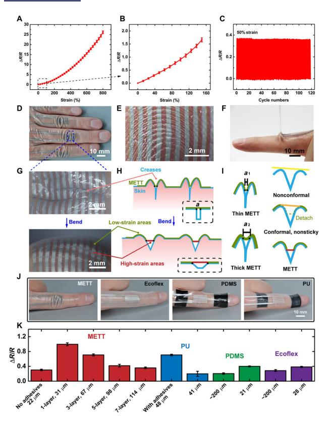
The METT is conformal and sticky, which can enable the crease amplification
