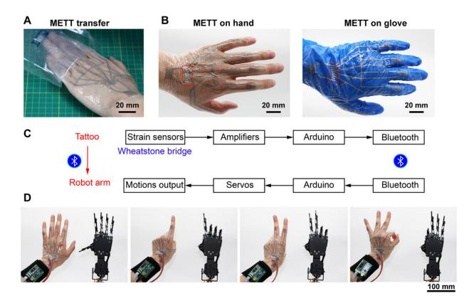
The METT can control the robotic hand remotely. (A) Photograph of transferring the tattoo onto the hand. (B) Photograph showing METT on the skin (left) and disposal glove (right). Dotted frame, the external contact pads. (C) System-level block diagram of the robot controlling system. (D) The METT can remotely control the movements of the robotic hand. Photo credit: Lixue Tang, Southern University of Science and Technology. Credit: Science Advances, doi: 10.1126/sciady.abe3778
