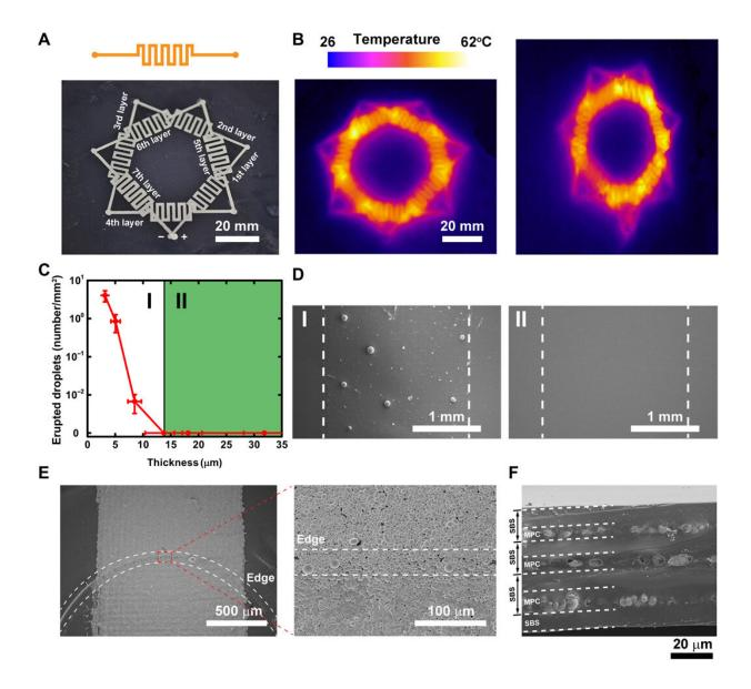
The scalability of the METT. (A) Optical image of the seven-layered heater. (B) The thermal image of the heater without deformation (left) and with 30% strain (right). (C) The numbers of the erupted liquid metal droplets depend on the thickness of the SBS layer after the stretch cycles. (D) Scanning electron microscopy (SEM) characterization of the surface of the SBS corresponding to (C); the thickness of the SBS in I (left) and II (right) is 4.8 and 18.13  $\mu$ m,
