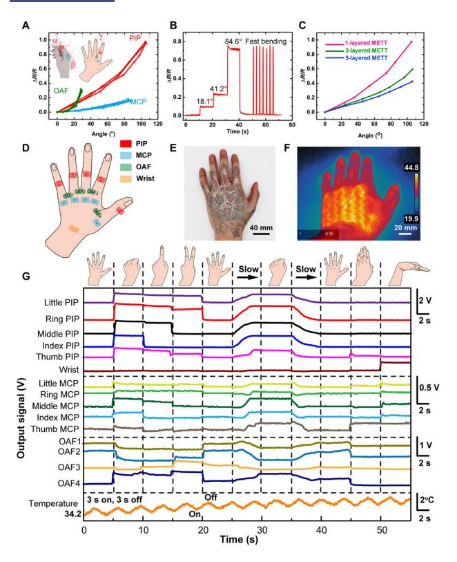
The METT can monitor the movements of the hand. (A)  $\Delta R/R$  of strain sensors in different position versus angles. Inset: The schematic illustration of the measurement positions of the strain sensors. (B) Resistance response of the
