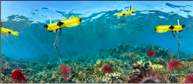
Image representing the use of multiple COTSbot AUVs for COTS control. Credit: Abbasi et al.
