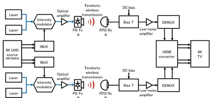
Block diagram of the 8K video wireless transmission system showing two 24-Gbit/s channels. Credit: Osaka University
