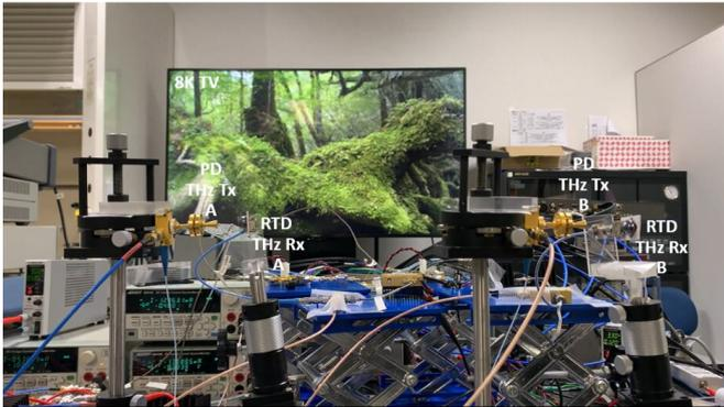
Photograph of the real-time 8K experiment. Foreground shows the two photodiode transmitters (Tx) and two resonant tunnelling diode receivers (Rx) with 8K television (TV) screen in the background. Credit: Osaka University
