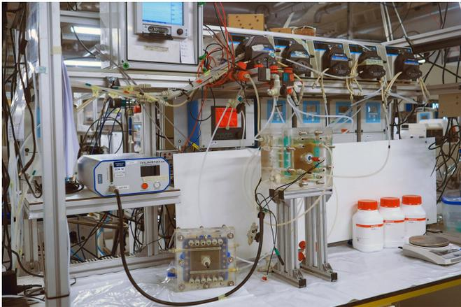
Lab-scale setup for capturing CO<sub>2</sub> from seawater. Through the transparent module in the center, where green square seals and brown membranes are visible, (artificial) seawater containing CO<sub>2</sub> flows, and the pH is successively lowered and raised, allowing the CO<sub>2</sub> to be separated. Surrounding this module are pumps, regulating valves, pH meters, and a power source to keep this process going and to accurately monitor it. Credit: TU Delft/Rose Sharifian
