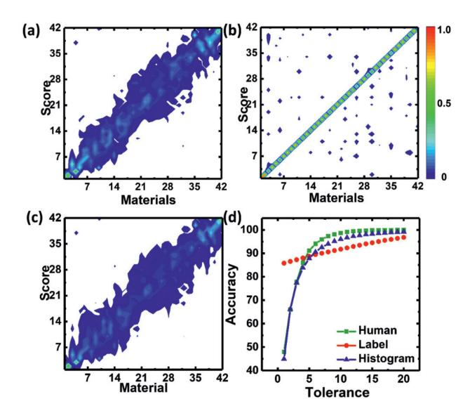
Deep learning for tactile decision-making. a) Histogram of human tactile cognition. b) Tactile histogram of the machine trained using labels. c) Output layer of the proposed histogram-based network for the 42 tactile materials with textures ranging from smooth/soft (bottom) to rough (top). d) Classification accuracy according to the tolerance bounds. Credit: Advanced Science, doi: 10.1002/advs.202002362
