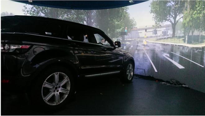
The WMG 3xD simulator, used to test the LiDAR sensors Credit: WMG, University of Warwick
